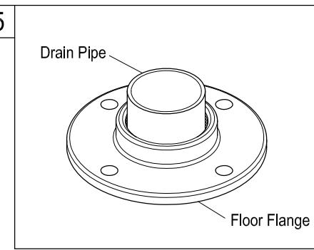
5. Secure floor flange to the area around the drain, this will serve as additional reinforcement to keep your tub drain in place in the event of any accidental impact on the tub.
