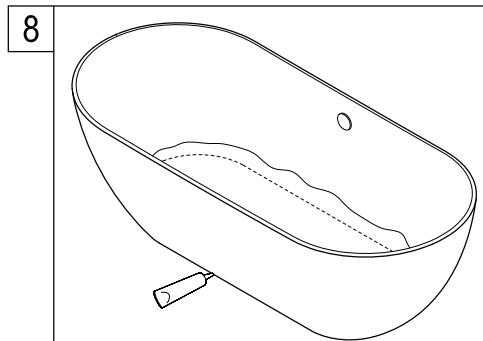
8. Close the drain and fill tub with 2" to 5" with water, while inspecting the connections from below the floor drain the tub and check for leaks. Apply caulking around the perimeter as needed, clean excess caulking.
