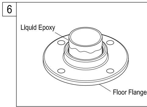
6. Apply liquid epoxy or a professional grade ABS glue or JB weld epoxy to the drain pipe coming from the floor, apply as per manufacturer's instructions.
