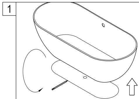
1. Position the tub at the desired location, with a pencil mark the perimeter of the tub, also mark the location of where the tub drain will be situated, remove tub and place upside down on a blanket or piece of cardboard.
