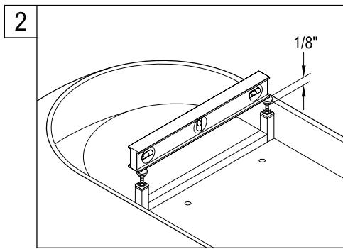
2. Adjust feet so that they protrude 1/8" below the level of the tub, you can accomplish this by placing a level or a straight piece of lumber across the width of the tub.
