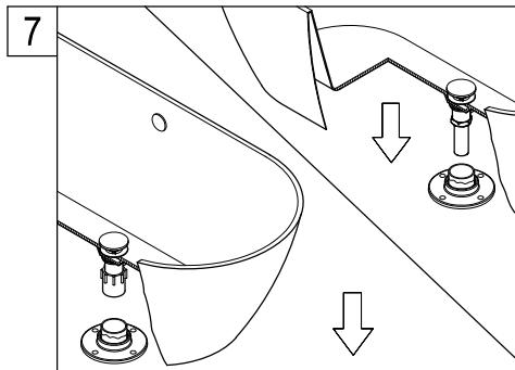
7. After Glue/ epoxy has been applied with the help of two or more people slowly pick up the tub and align the tub drain adapter to the drainage pipe, set tub in place.
