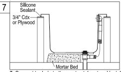
7. Connect to drain to the waste stub out and install faucet, fill the tub with water and check for leaks.
