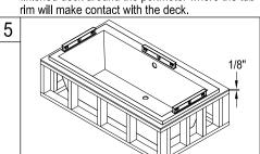
5. Set the tub on the mortar bed, making sure that the 1/8" thick shims are positioned around the perimeter of the tub and level the tub in all directions.
