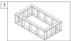
Build a recess deck to the specific measurements of your tub using 2" x 4" lumber.
