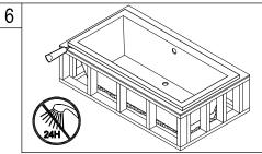
6. Let the mortar bed dry for at least 24 hours, check to make sure that all parts of the tub are adequately supported by the mortar bed, if necessary add mortar to the areas where the tub does not feel firmly supported, remove the shims and apply silicone caulking around the perimeter of the tub.
