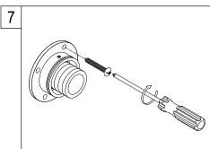
7. Screw the mounting plate to the wall with the mounting screws.
