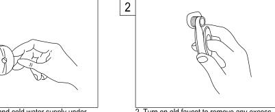
2. Turn on old faucet to remove any excess water in the supply lines. Apply Teflon tape onto the threads of supply elbow.
