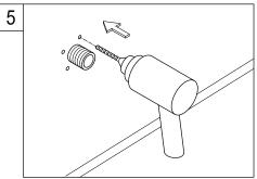
5. Drill holes at the marked locations and remove mounting plate from faucet body.
