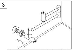
3. Insert mounting plate into the faucet body and install to water outlet on wall.
