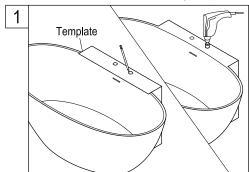
1. Drill holes for your deck mounted faucet by placing the attached template on top of the deck, this template is premeasured for a 7" center to center faucet requiring 2 holes only, if your faucet requires the drilling of additional holes or a different center to center dimension, please adjust accordingly.
