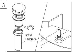
3. If you have access to the tub drain from below the floor, apply Teflon tape to the drain and thread the included tailpiece, measure the distance that it protrudes from the bottom of the tub and rough in your drain pipe accordingly.
