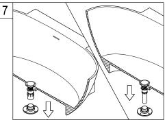
7. After Glue/ epoxy has been applied with the help of two or more people slowly pick up the tub and align the tub drain adapter to the drainage pipe, set tub in place.
