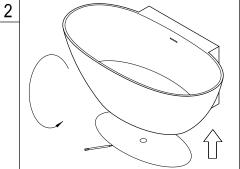
2. Position the tub at the desired location, with a pencil mark the perimeter of the tub, also mark the location of where the tub drain will be situated, remove tub and place upside down on a blanket or piece of cardboard.
