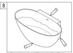
8. Close the drain and fill tub with 2" to 5" with water, while inspecting the connections from below the floor drain the tub and check for leaks. Apply caulking around the perimeter as needed, clean excess caulking.
