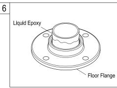
Apply liquid epoxy or a professional grade ABS glue or JB weld epoxy to the drain pipe coming from the floor, apply as per manufacturer's instructions.
