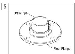
5. Secure floor flange to the area around the drain, this will serve as additional reinforcement to keep your tub drain in place in the event of any accidental impact on the tub.
