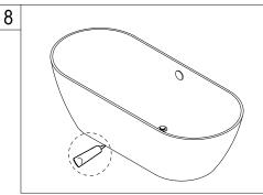
8. With the bathtub now in place, wipe off any excess tub and tile caulk and adhesive where the tub meets the floor. Run a bead of tub and tile caulk around the bottom edge of the bathtub where it meets the floor.
