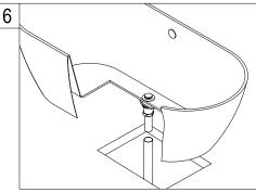
6. Carefully set tub into position and connect the drain hardware (previously installed). Finish the installation of the tailpiece installation.
