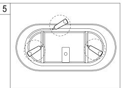
5. Apply a generous bead of adhesive or silicone to the bottom of the tub supports. Then apply a bead of tub and tile caulk around the edge of the base.
