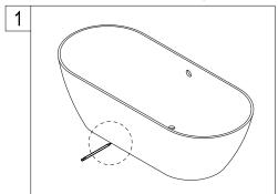
1. Clean, level, and prepare the floor for installation. Place the unit in the exact installed position on the floor and trace the outline of the bath with a pencil or any erasable marking.
