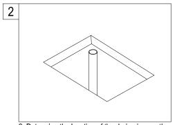
2. Determine the location of the drain pipe, on the floor by taking measurements of the drain and waste location underneath the unit.
