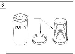
3. Clean the drain hole area in preparation of setting the drain. The area should be dry and free of any debris. Apply a bead of clear silicone or plumbers putty around the Drain Body and pass it through the drain hole. Apply plumbers putty to the Washer and slide it over the bottom of the drain body.
