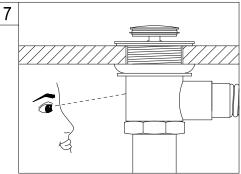
7. Fill the tub with water to the overflow and then drain the tub while inspecting the waste connections below the floor for leaks. Access from below will be necessary for this step.
