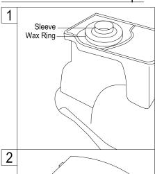
1. Set the bowl upside down on a soft surface Press the wax ring onto the toilet bottom outlet, remove the rag from the drain opening.
