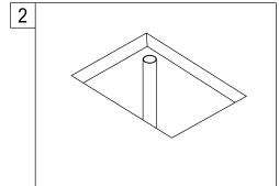
2. Determine the location of the drain pipe, on the floor by taking measurements of the drain and waste location underneath the unit.
