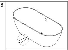
8. With the bathtub now in place, wipe off any excess tub and tile caulk and adhesive where the tub meets the floor. Run a bead of tub and tile caulk around the bottom edge of the bathtub where it meets the floor. Wipe off any excess caulk with a wet cloth.
