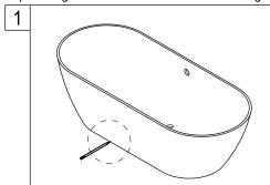
1. Clean, level, and prepare the floor for installation. Place the unit in the exact installed position on the floor and trace the outline of the bath with a pencil or any erasable marking.
