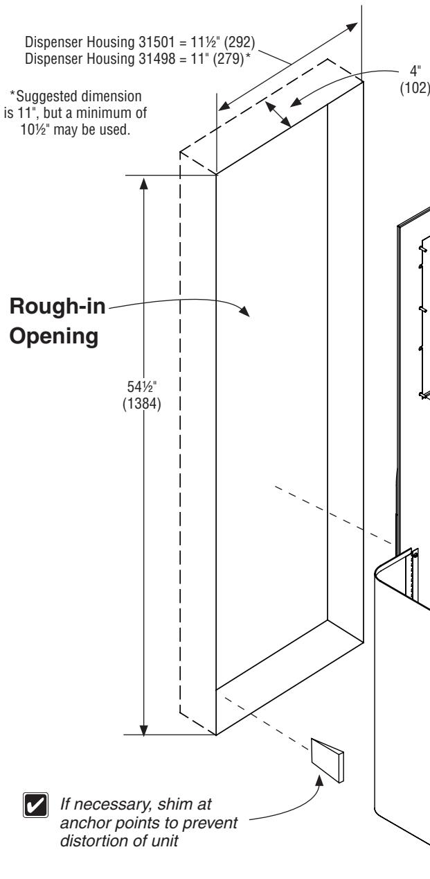
Use (4) Screws (not included) and (6) Nylon Thumb Nuts (included) to mount dispenser housing and stainless steel wall unit into the rough-in opening.
