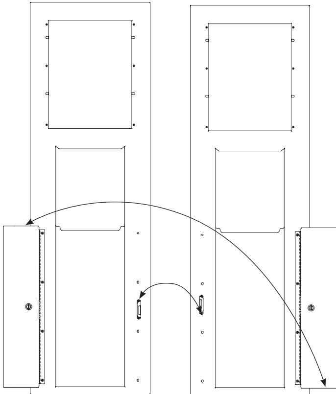
*Rotate door and lock 180° to reverse swing direction of door.*
