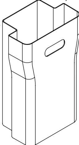
If necessary, shim at anchor points to prevent distortion of unit
