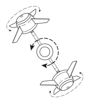
Both fan heads have 3 forward speeds and manual reverse. Both fan heads can also rotate around the central fan body. The reverse button on the wall control serves as on/off for the central body rotation.
