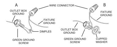
8) Make wire connections. Reference chart below for correct connections and wire accordingly.
