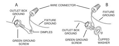
Make wire connections. Reference chart below for correct connections and wire accordingly.
