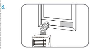
Insert the window slider adaptor into the hole of the window slider.
