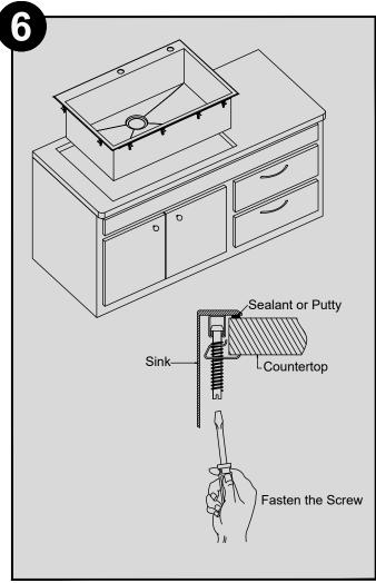
Insert the sink into the opening, check the alignment of the sink to the cutout in the countertop and press firmly. Tighten the screws in the front of the sink, followed by the ones in the back and on the sides of the sink. Remove any excess silicone-based sealant. Allow the sealant to set for 30-60 minutes.
