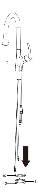
1. Remove the mounting nut (#11), rubber&metal washer (#10) from the faucet body (#2).
