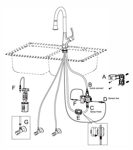
A. Fix the control box holder to the wall with the screws provided (part A in the picture). Then attached the control box to the holder.
