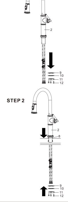
1. Remove the mounting nut (#11), clamp (#10) and rubber washer (#9) from the faucet body (#2).
