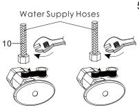
5. Apply Teflon tape onto the threads of the faucet water supplies in a clockwise direction. Tighten the water supply tubes onto the water supply shut offs. Be sure to connect the cold water supply tube to the cold water supply valve (typically on the right) and the hot water supply tube to the hot water supply valve (typically on the left). Use a wrench (as shown) to tighten the nut.
