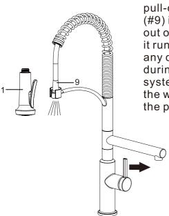
6. Unscrew the spray head (#1) from the pull-out hose (#9). Hold the pull-out hose (#9) in the sink to avoid spraying water out of the sink. Turn on the water and let it run for one minute. This will help clear any debris that may have come loose during installation and prevent the system from becoming clogged. Turn off the water, screw the spray head (#1) onto the pull-out hose(#9).
