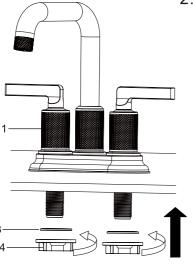
2.From under the sink, secure the faucet with washers(#3) and mounting nuts (#4).Tighten the lock nut by hand. Do not over tighten!
