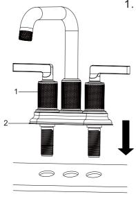
1. Place the faucet body (#1) and gasket (#2) on top of the sink and insert through the installation holes.
