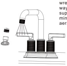
4. Remove the aerator using the aerator wrench. Turn the faucet handle all the way on, turn on hot and cold water supply and flush water lines for one minute. Reinstall aerator using the aerator wrench.
