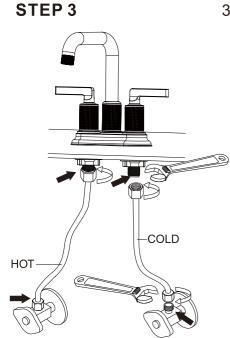
3. Connect the water supply lines to the tail pipes of the faucet and to the hot and cold water supply valves. Secure and tighten with an adjustable wrench. Caution: Be careful not to mix up the hot and cold supply lines. Check all connections (shown with arrows in the image) for leaks. Re-tighten if necessary. Do not over tighten!
