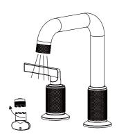
4. Remove the aerator with an aerator wrench. Turn the faucet handle all the way on, turn on the hot and cold water supply and flush water lines for one minute. Reinstall the aerator with an aerator wrench.
