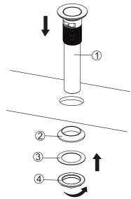
3. From the top of the drain hole, place the drain ① through the installation hole. From under the drain hole, install the thick washer ② ,washer ③ and nut ④ by hand twisting on to the tail pipe of the drain. Then, install the tail pipe to the wall plumbing. Use of plumbers putty or silicone is recommended to seal drain ① to top side of bowl.
