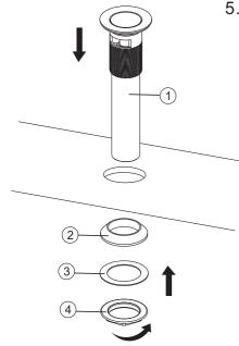
5. From the top of the drain hole, place the drain ① through the installation hole. From under the drain hole, install the thick washer ②, washer ③ and nut ④ by hand twisting on to the tail pipe of the drain. Then, install the tail pipe to the wall plumbing.
