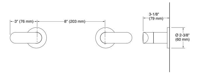
Technical Information All product dimensions are nominal. Drain included: No Notes Install this product according to the installation guide. ADA, OBC, CSA B651 compliant when installed to the specific requirements of these regulations.
