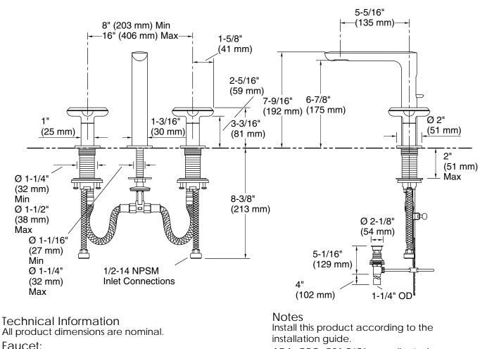
ADA, OBC, CSA B651 compliant when installed to the specific requirements of these regulations.
