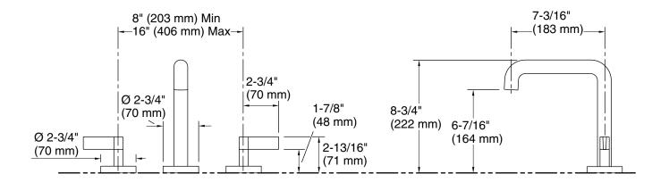
Technical InformationAll product dimensions are nominal.Faucet:Flow rate:9.98 gal/min (37.8 l/min)Pressure:45 psi (3.1 bar)Drain included:NoSpout:Spout reach:7-3/16" (183 mm)
