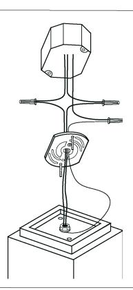
Tuck wires and wire nuts into junction box.
