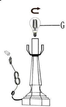
Step 1 Insert the bulb(G) into the socket(C).
