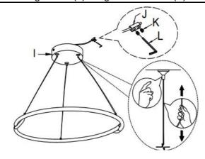
**Step 4**: Press the expansion piece and adjust the height of the lamp body(I). If the expansion piece fails, Move wire locking device(J) to the desired position and lock it with hex screw (K) and allen wrench (L).
