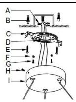
**Step 3**: Carefully remove packaging from fixture, adjust wire length to desired mounting height, fix the lamp body (I) to mounting bracket(C) using machine screw(H).
