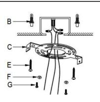
**Step1**: Punch the hole and install the Wall plug (B) to the ceiling. Fix the mounting bracket (C) to the outlet box with tapping screw (E) and mounting screw (G).
