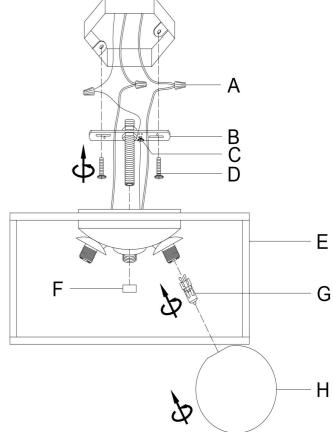
PLEASE USE ON/OFF TYPE "G9" BULB MAX 25-WATT OR LED BULB MAX 5 -WATT THERE ARE 3PC 3-WATT BULB IN THE BOX
