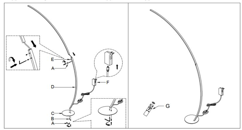
3.Insert transformer (F) correctly.4.Adjust the lights with the remote control (G).
