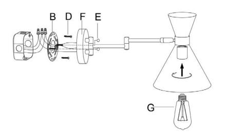
Step 3: Fix the lamp body (F) to the mounting plate (B) with nuts (E). Then Step 4: You can adjust the lampshade left and right, up down. insert the bulb (G) into the lamp body (F).
