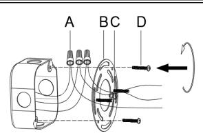
Step 1:Connect the mounting plate (B) to the junction box using the mounting screws (D).
