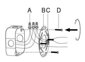
Step 1:Connect the mounting plate (B) to the junction box using the mounting screws (D).
