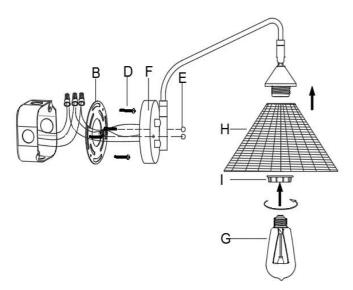
Step 3: Fix the lamp body (F) to the mounting plate (B) with nuts (E). lock the shade (I) with a socket ring to the Lamp Body (F), and then insert the bulb (G) into the lamp body (F).
