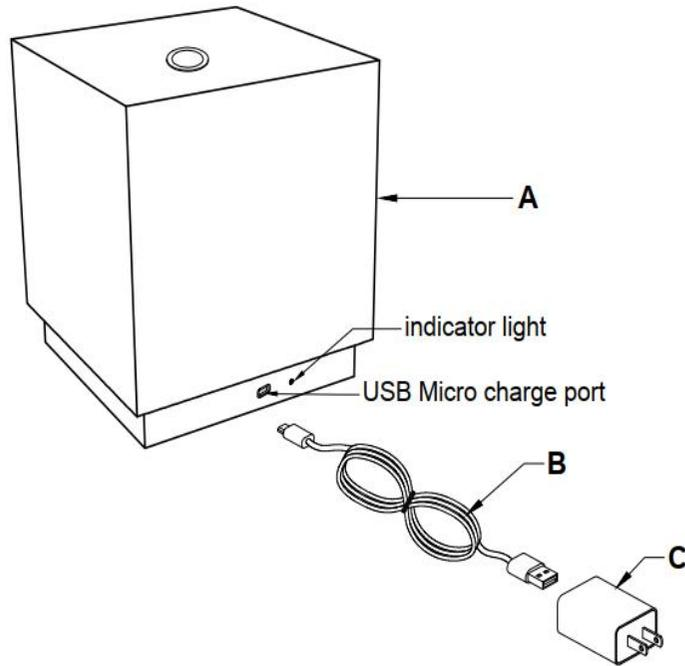
1. One end of charging cable (B) is connected to lamp body (A) USB Micro charge port and the other end is connected to Charging plug (C).
