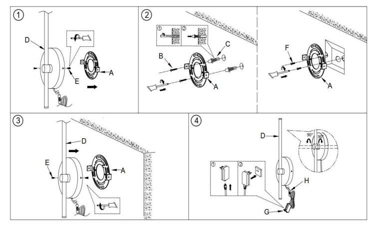
3.Fix the lamp body (D) on the mounting bracket (A) with the mounting screw (E)4.Connect plug (G) to lamp body (D) and adjust lamp body. Insert plug (G) into the power outlet and adjust the light source with dimmer switch (H). Complete the installation.
