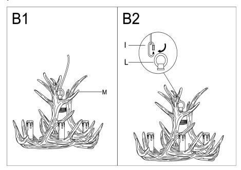
Step B1: Open the quick links (I) to connect the loops (L) on the antler chandelier main body(M), and to connect the loop(L) Close the quick links(I)
