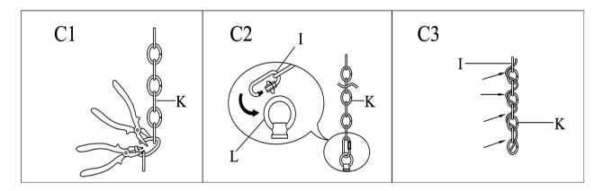
Step C1: By measuring, determine the correct length of links needed. Use the chain pliers, open and discard the remaining chain.
