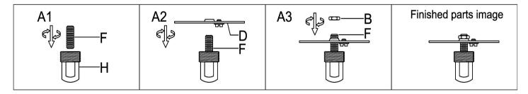
Step A1:Thread the nipple(F) into the screw collar loop(H)
