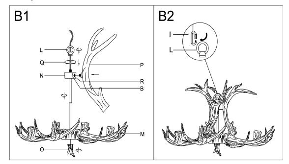
Step B1: Separated trim(N) from loop(L) round iron plate (Q).
