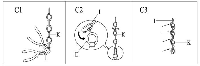
Step C1: By measuring, determine the correct length of links needed. Use the chain pliers, open and discard the remaining chain.
