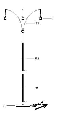
Screw the Lamp body (B3) onto the Lamp body (B2)
