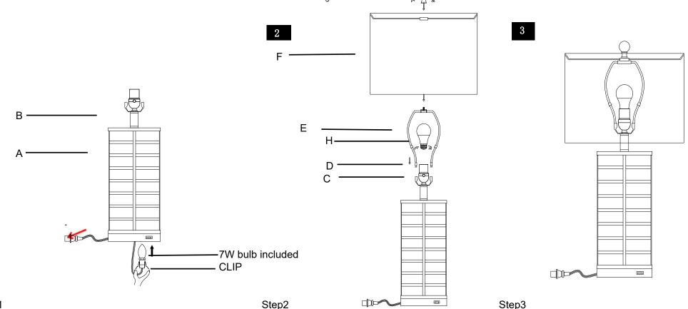
Step 1 Pinch the clip from base Replace with 7W bulb(bulb included) Put the clip back carefully and not twist the cord
