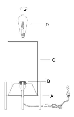
Step 1 Insert the bulb(D) into the socket(B).
