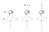
3. Fix the mounting bracket(B) to the outlet box with machine screw(C).
