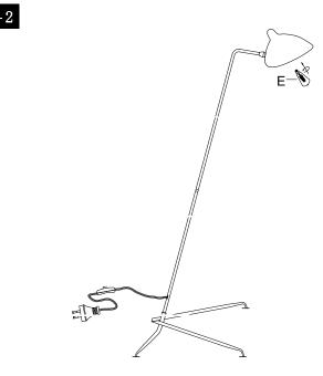
Step 2 Insert the bulb(E) into the socket. Put the light on a level surface to check if everything is stable.
