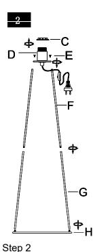
Unscrew the Socket Ring(C) and Screw (E)from the Socket Assembly(D).
