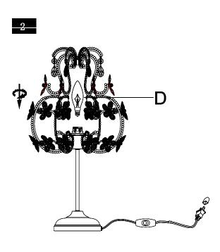
Step 2 Insert the bulb(D) into the socket.
