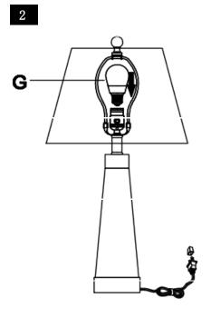
Step2 Insert the bulb( G) into the socket(C).
