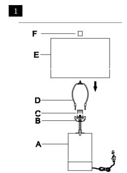
Step 1 Insert the Harp (D) into the Saddle (B). Put the shade(E) on the Harp(D), then tighten the Finial (F)into the Harp (D)
