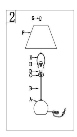
Step 2 Put the shade(F) on the Harp(E), then tighten the Finial (G)into the Harp (E) Insert the bulb(H) into the socket(D).
