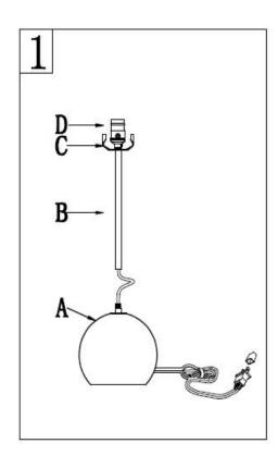
Step 1 Pull power cord to connect the Lamp Body (B) to the Base (A). Insert the Harp (E) into the Saddle (C). Screw the Lamp body (B) onto the Lamp base(A) Be careful not to twist the power cord and tighten securely
