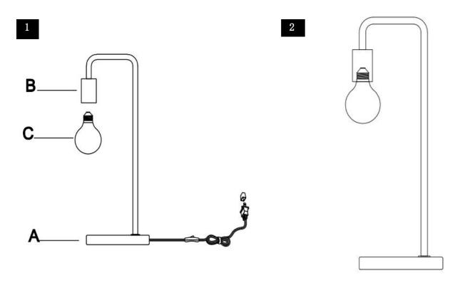
Step 1 Insert the bulb (C) into the socket (B).
