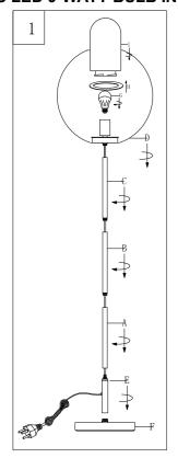
Step 1 Make sure all parts could be aligned before assemble Do not rotate lamp body too hard avoid base screw broken Put the silicone strap(H) on the waterproof shade(I), Screw the tube (E) onto the Lamp base (F)
