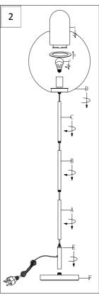
Step 2 Insert the bulb(G) into the socket. then tighten the Finial into the socket base.
