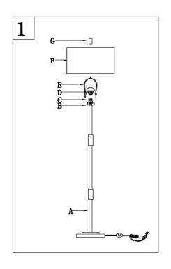
Step 1 Insert the harp (D) into the saddle (B). Put the shade(E) on the harp(D), then tighten the finial (F)into the harp (D) Insert the bulb(G) into the socket(C).
