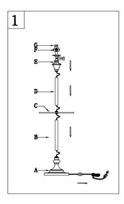
Step 1 Make sure all parts could be aligned before assemble Do not rotate lamp body too hard avoid base screw broken Screw the Lamp body (E) onto the Tube(D)
