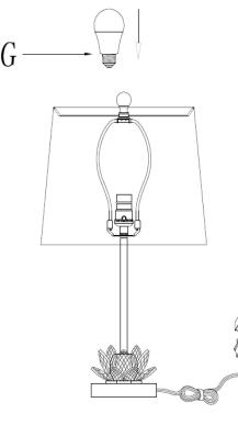
Step2 Insert the bulb(G) into the socket(C).
