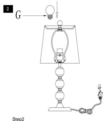
Insert the bulb(G) into the socket(C).
