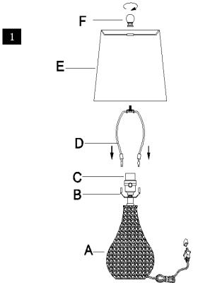
Step 1 Insert the Harp (D) into the Saddle (B). Put the shade(E) on the Harp(D), then tighten the Finial (F)into the Harp (D)
